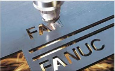
CNC lasers - reliable sheet metal separation FANUC CO2 laser with 2-D and 3-D cutting technology
