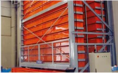
Automated warehouses for vertical stocking of plate sheets
