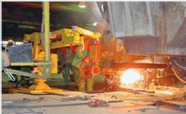
Pneumatic manipulator with gripping jaws for picking and handling casting moulds
